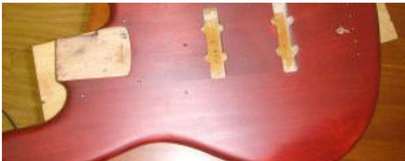
After another paint-and-wipe process of the nashiji-urushi solution diluted with turpentine, apply the paint-and-wipe process a few more times but this time with colored urushi. This seems similar to the see-through painting process, but the process is quite different because the wipe lacquering requires painting multiple times. These processes may be the main feature to create the beautiful texture that is unique to the wipe-lacquered guitar.
