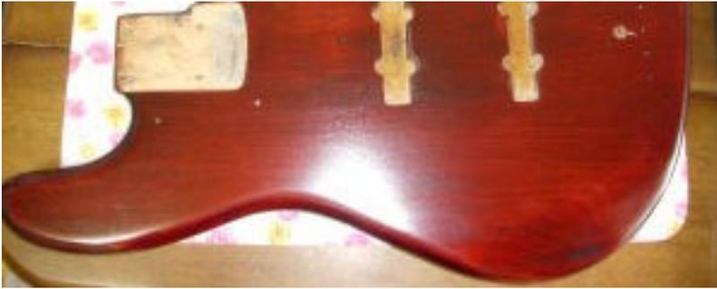
After repeating the paint-and-wipe process for about 10 times. From this point, we use soft paper instead of cloth to have some amounts of lacquer remain on the surface to give the body a nice gloss.
