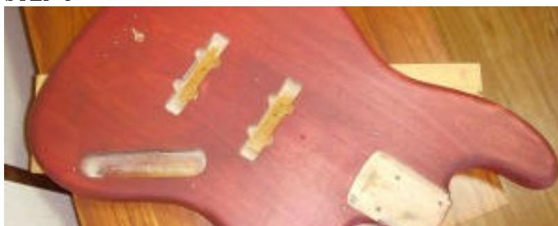
After the first paint-and-wipe process and coloring, the body is dried in a high-humidity drying closet called *urushi-buro* or lacquer bath. The temperature inside the closet is maintained between 20-25 degrees C (68-77 degrees F) and the humidity between 75-85%. The laccase enzyme contained in urushiol, an oil content of the urushi sap, reacts with oxide and moisture content in the atmosphere to form polymer resin and solidifies urushiol.
