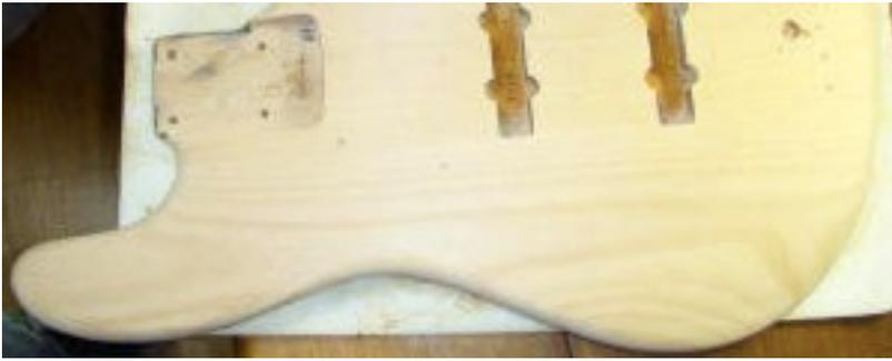
First, scrape the existing paint using an electronic sander. In order to remove the polyester coat, which is almost penetrating into the wood, use force and forget about some small scars you may have to leave with the sander. Our veteran craftworkers then polish the surface carefully to erase the scars.
